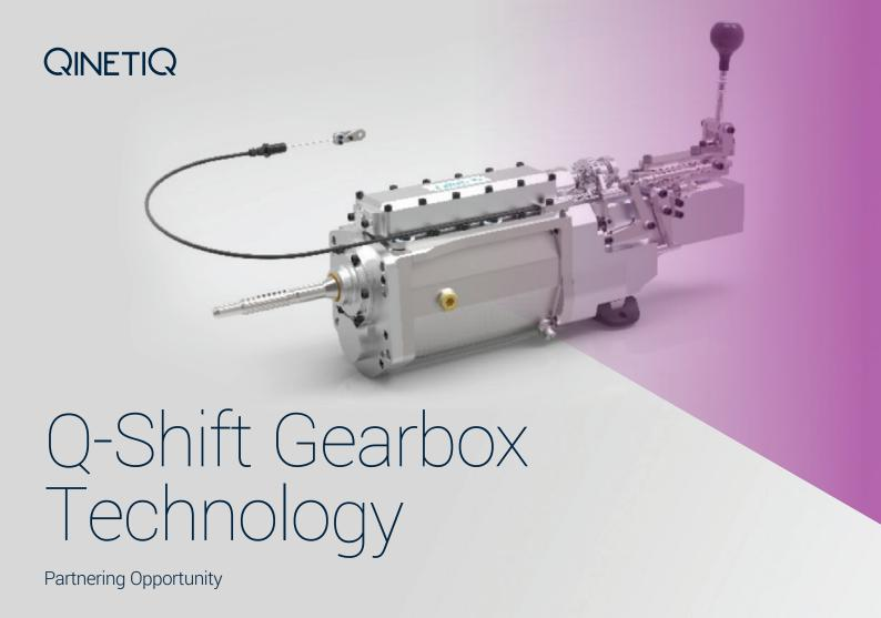
Q-Shift is a high performance low cost gear change technology. It uses simple dog clutch components to pass the driving torque directly from one gear to the next, without passing through a neutral state. Its sequential shift event is controlled mechanically via a simple barrel arrangement. Additional patents in the portfolio take this concept further, including a version which seamlessly multiplies the number of ratios.
