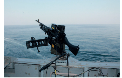
POINTER Optical Sight integrated with General Purpose Machine Gun
