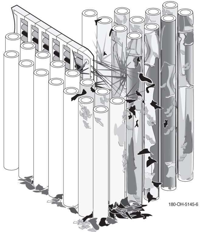
Figure 1: CECIL's shadow zone lance effectively removes soft sludge from as tube lands and shadow zones between tube lanes
