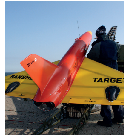
The Banshee target can simulate an enemy aircraft or cruise missile
